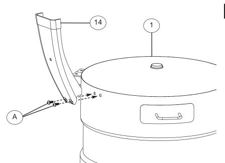
Attach leg (14) to outer shell (1) using pan head screws (A) as shown.
